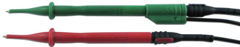
Fig 3. Prods in 2 wire testing configuration
